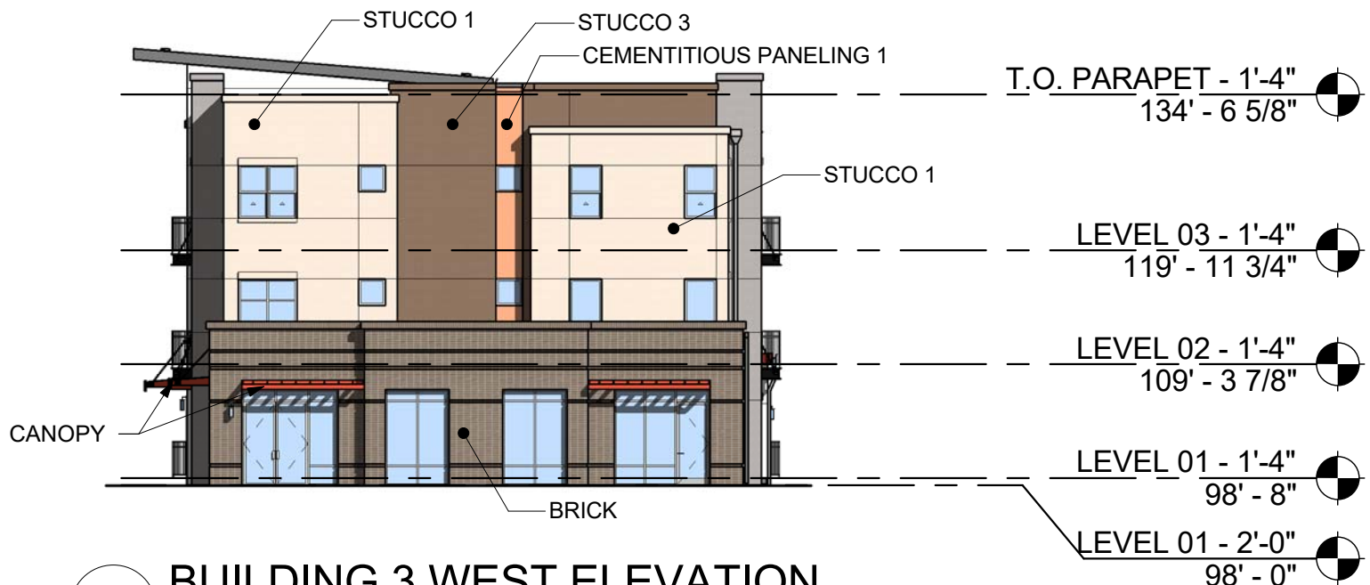
4 BUILDING 3 WEST ELEVATION SCALE: 1/16" = 1'-0"
