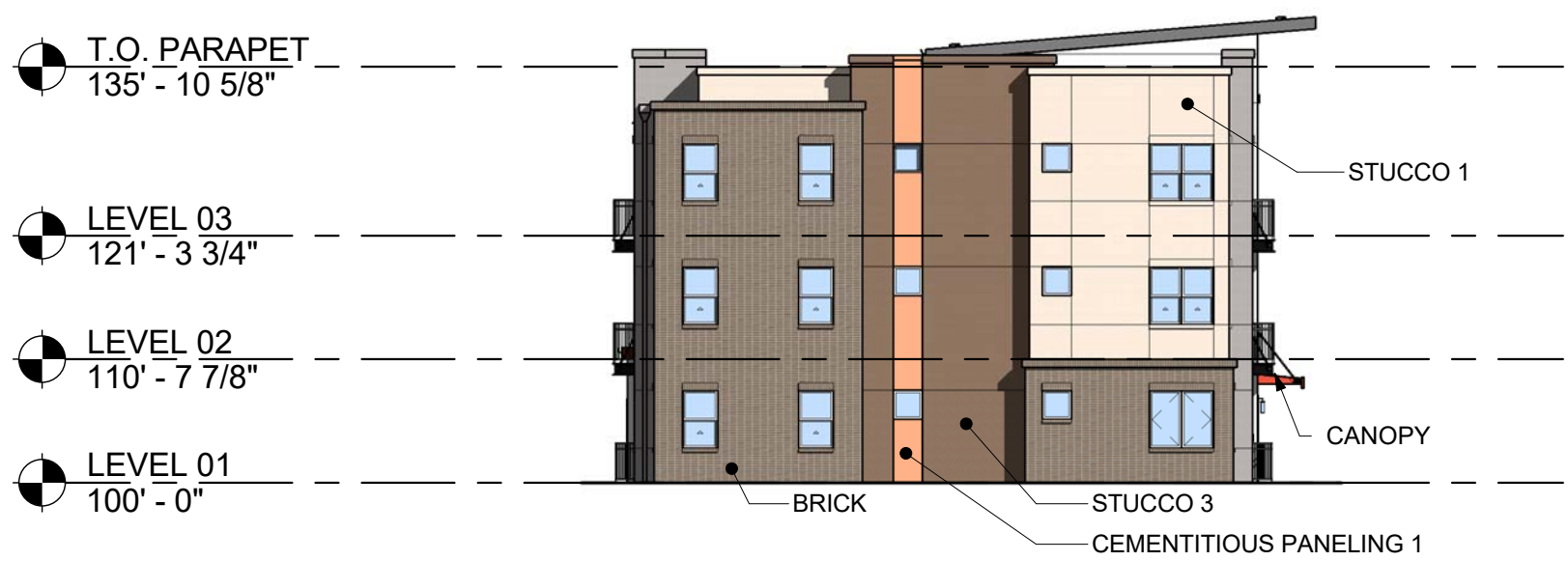
3 BUILDING 3 EAST ELEVATION SCALE: 1/16" = 1'-0"
