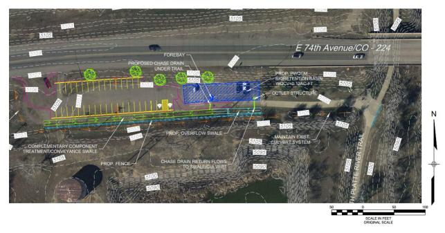
The vegetated bioswale located south of the Engineer's Lake Trailhead Parking Lot will collect sheet flow and direct flows to the new bioretention basin prior to releasing back into the existing east-west drainage ditch. The project will treat a portion of CDOT MS4 area on SH 224A which is not currently being treated prior to discharging to the South Platte River. The bioretention basin will be constructed within the 100-yr floodplain but outside the floodway.
