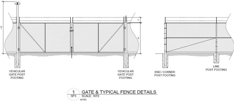
1. FENCE WILL BE GALVANIZED CHAIN LINK WITH 2" MESH, 9 GAUGE.
